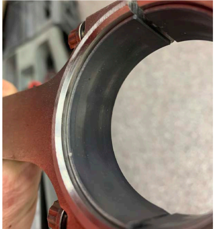
These main and rod bearings treated with dry film coating show excellent bearing protection after 13 years of service in a 180HP VW engine. Note that the rod bearings have yet to wear through the sacrificial coating, and the mains only show some wear that indicates debris had contaminated the engine oil at some point during the 13 years of service.
