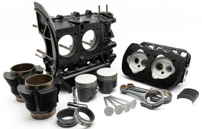
Engine components for “Project 1385” after receiving a full complement of thermal barrier, thermal dispersant, and friction reduction coatings.
