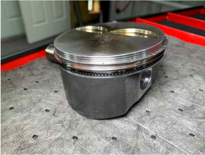
Dry film coated piston skirt after 69 hours of dyno test time, still looks new.
